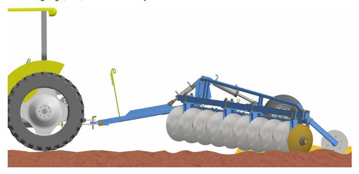
• On both cases, from the third and forth pass on, the hydraulic cylinder should be activated a little more, where it can be notice the actuation of all disc blades.
