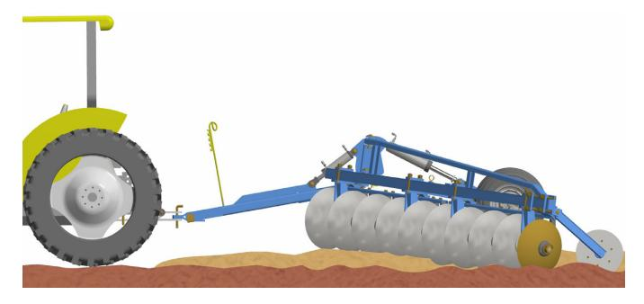
• On the other passes, gradually activate the hydraulic cylinder until the conclusion of the terrace, which will be ready from 10 to 12 passes on average.
